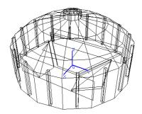
For this part of exercise a room has been prepared for you. It is actually a model of an old gas container, which has been transferred into a theatre. The geometry has been defined, materials have been selected and a point source has been defined. The source has been assigned the Omni directivity pattern and the sound power of the source to 31 dB. This means that the source is calibrated to give 0 dB SPL (sound pressure level) at a distance of 10 m in a free field
