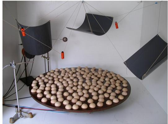
**Figure 4:** Measurement of the random incidence scattering coefficient. Left: principle. Right: A 1:5 scale reverberation room with the measurement setup. (Ref.: Vorländer et al. (2004)).
