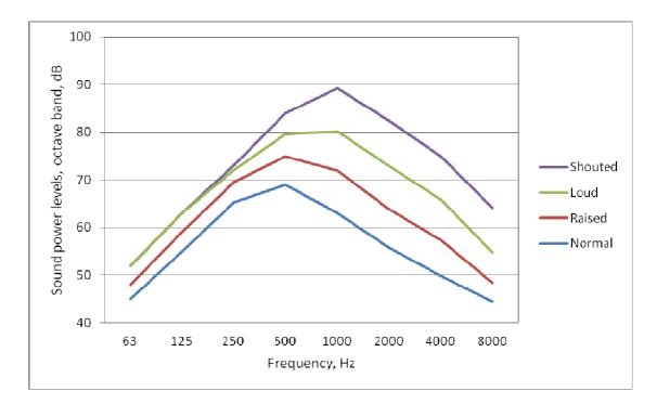
*Fig. 1 – Speech spectra in octave bands for different vocal effort. Data at 250 Hz and above are from ANSI 3.5 [5], values below 250 Hz are suggested based on measurements presented in this paper.*
