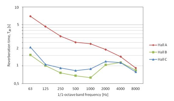
Fig. 5 – Measured reverberation time  $T_{20}$  in octave bands in each of the three halls.
