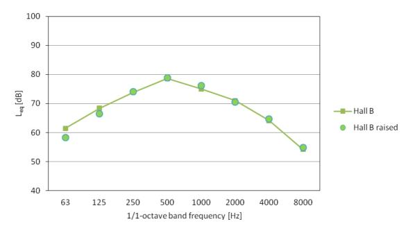
*Fig.* 8 – *Measured and predicted noise spectra in hall B. Calculations were made with 'Raised' speech spectrum.*
