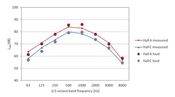
Fig. 7 – Measured and predicted noise spectra in hall A and C. Calculations were made with 'Loud' speech spectrum.
