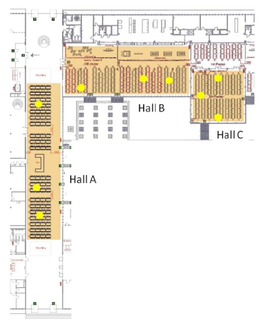
Fig. 3 – The three halls with table plans. The three microphone positions in each hall are marked in yellow.
