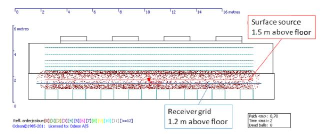
*Fig.* 2 – *Section of Hall C showing the position of surface source and receiver grid. The picture shows also emission of sound particles 2 ms after start.*
