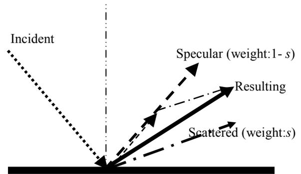
Figure 3: Vector based scattering. Reflecting a ray from a surface with a scattering coefficient of 50% results in a reflected direction which is the geometrical average of the specular direction and a random (scattered) direction. Note: Scattering is a 3D phenomena, but here shown in 2D.
