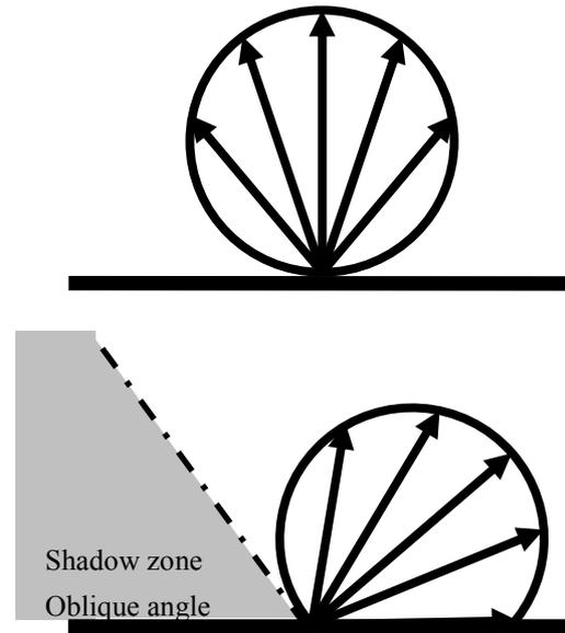
Figure 6: Traditional Lambert directivity at the top and Oblique Lambert at the bottom. Oblique Lambert produces a shadow zone where no sound is reflected. The shadow zone is small if scattering is high or if the incident direction is perpendicular to the wall. On the other hand if scattering is low and the incident direction is oblique then the shadow zone becomes large.
