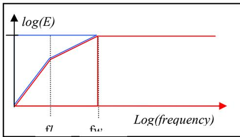
Figure 5: Energy reflected from a free suspended surface given the dimensions  $l \cdot w$ . At high frequencies the surface reflects energy specularly (red), at low frequencies, energy is assumed to be scattered (blue).  $f_w$  is the upper specular cut off frequency defined by the shortest dimension of the surface,  $f_l$  is the lower cutoff frequency which is defined by the length of the surface.
