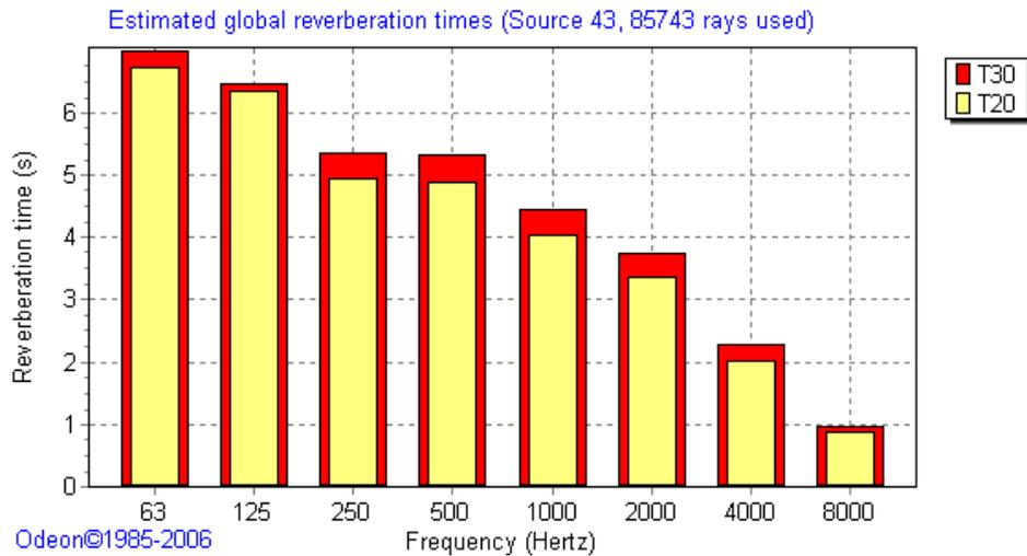
Figure 6: Reverberation times  $T_{30}$  and  $T_{20}$  derived from the global decay curves in Fig. 5.
