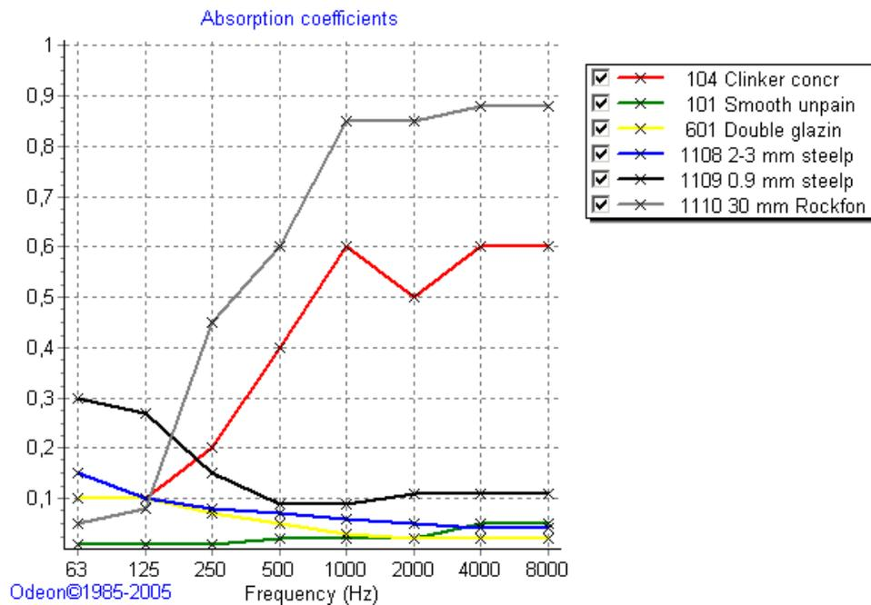
Figure 4: Absorption coefficients of the surfaces as used in the model.
