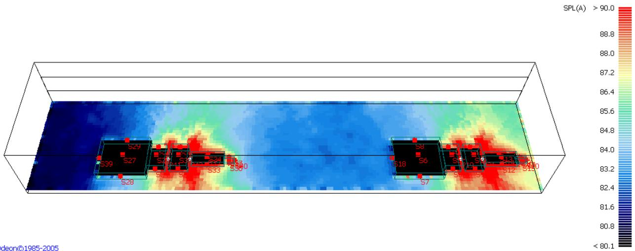
Figure 10: Mapping of the A-weighted sound pressure level with both turbines active. The grid size is 1 m and the height is 1.5 m above the floor.
