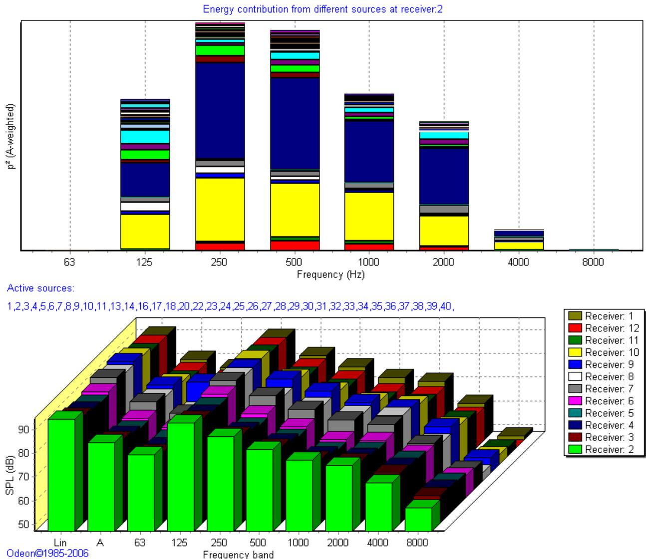
Figure 11: Above - Analysis of the sound sources' contribution to the sound energy in receiver 2. Below - Display of the sound pressure level (Linear, A-weighted and eight octave bands) in the 12 receiver positions.
