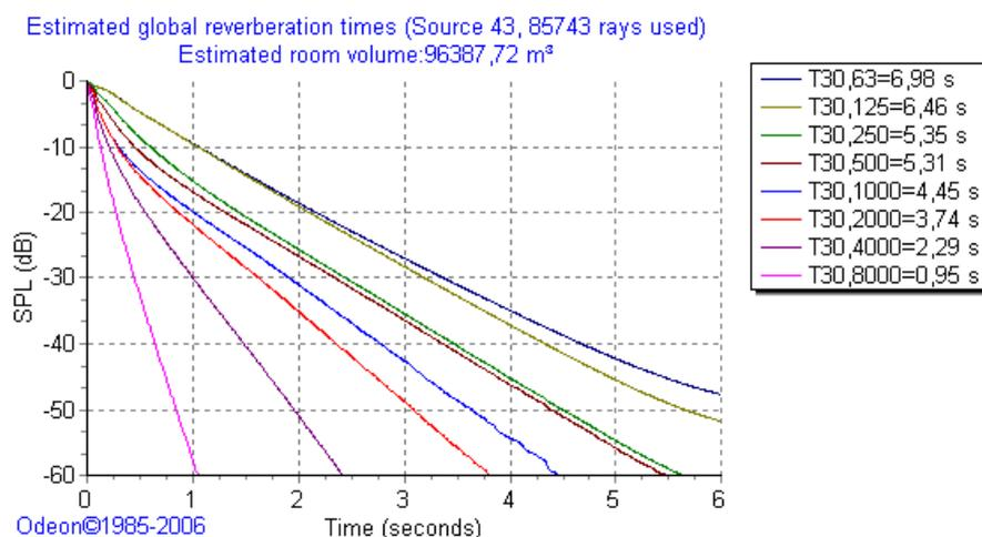
Figure 5: Global decay curves calculated for eight octave bands. The derived reverberation times are listed in the box to the right
