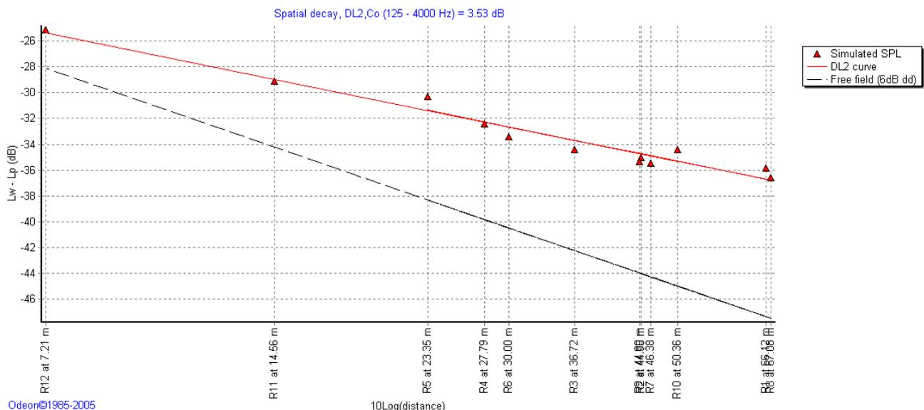
Figure 7: The spatial decay curve calculated for the omni-directional source and the 12 receivers shown in Fig. 3. The frequency averaged slope is  $DL_2 = 3.53$  dB per distance doubling.
