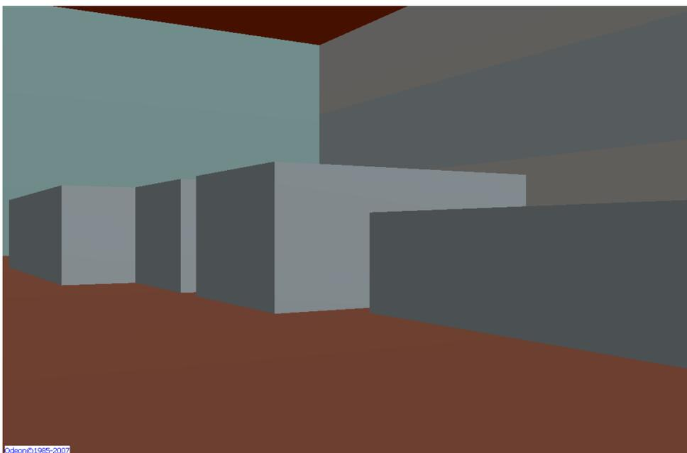
*Figure 2: A view into the acoustical model of the turbine hall. The colours indicate different absorption data for the surfaces.*
