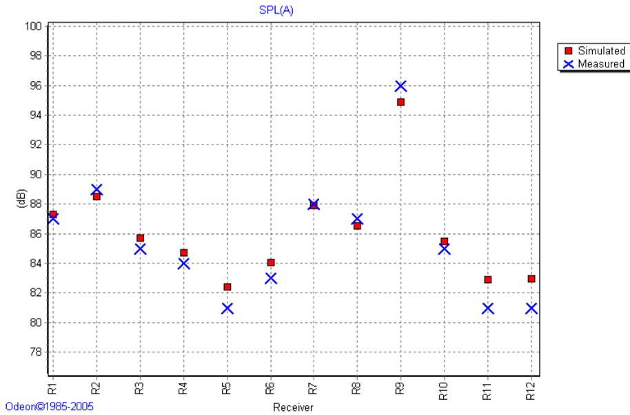
Figure 9: Comparison of calculated and measured A-weighted sound pressure levels in the 12 receiver positions.
