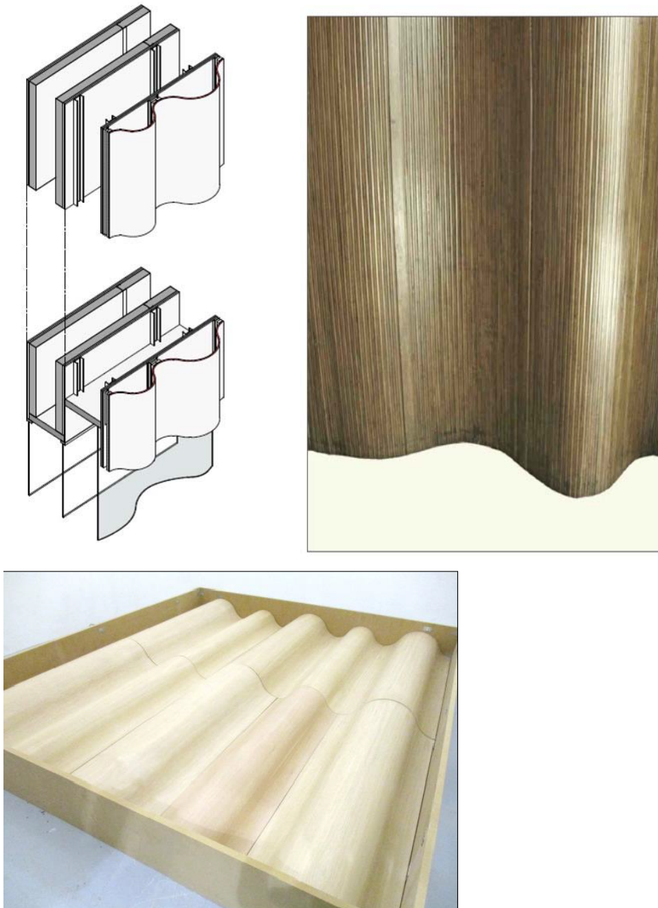
Figure 5 - Sound diffusing/curved solid wood panels, 218-270 mm cavity (Courtesy of estudio Herreros).
