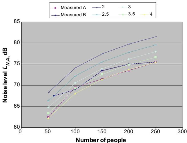
Fig. 3. Measured and predicted noise level for a canteen [3] (1235 m<sup>3</sup>) as a function of the number of people present. Measurement A: first period with increasing number of people; Measurement B: second period with decreasing number of people. The parameter on the predicted curves is the assumed group size, *g*.
