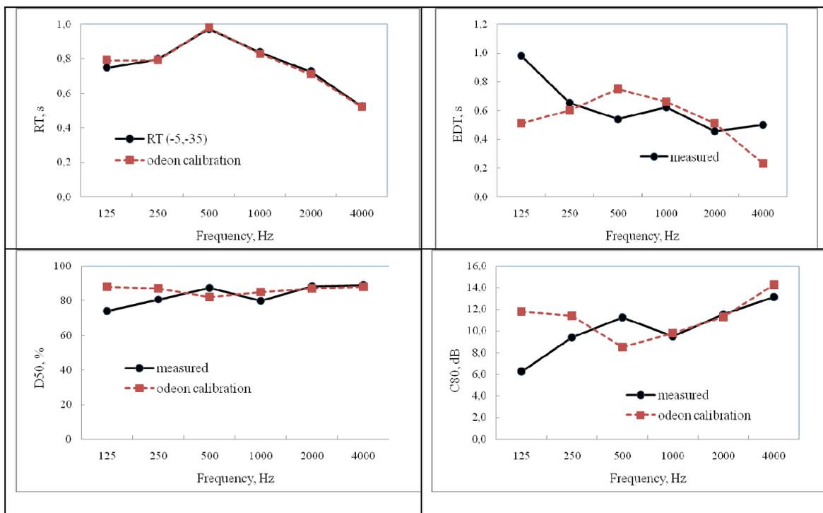
Figure 4 – Average acoustic parameters in according to ISO 3382 (RT, EDT D50 and C80). Measured (black line ) versus numerical calculation (red line) values.
