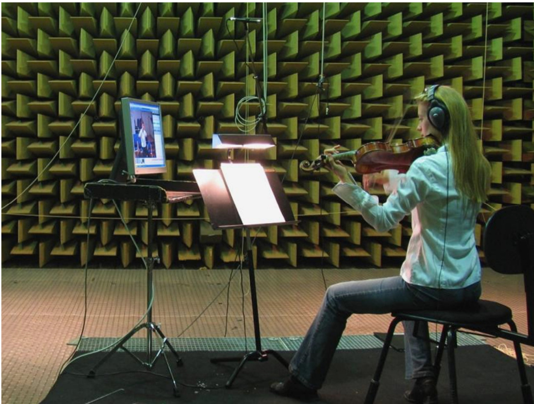
Figure 1. Recording of a violin part in the anechoic room at DTU. The conductor appears on the monitor and the sound of the orchestra in the headphones.
