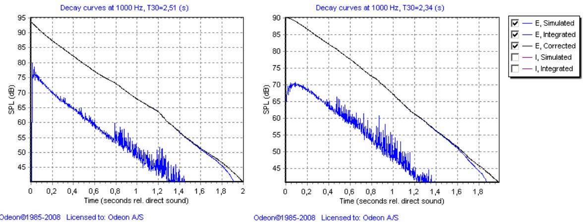
Figure 2. Calculated decay curves and integrated squared impulse response curves.
