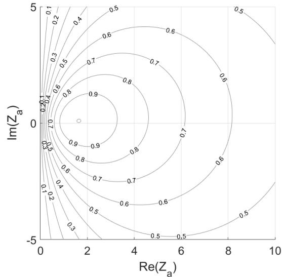
Figure 1 – Iso-absorption coefficient for  $ke = 60$  according to Eq. (1)
