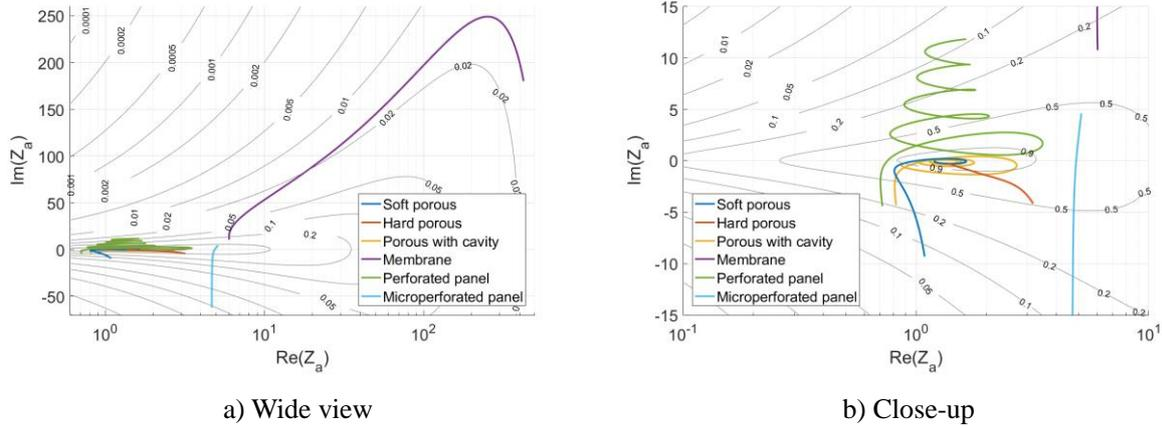
Figure 2 – Surface impedances of the test cases
