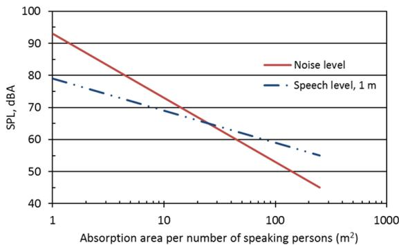
Figure 1. Ambient noise and vocal effort as functions of absorption area per number of speaking persons.
