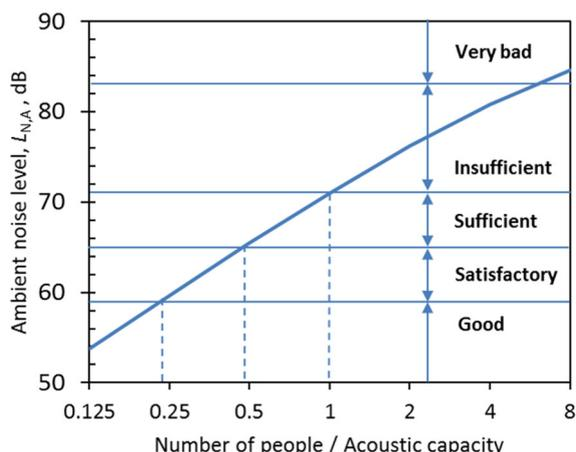
Figure 3. Ambient noise level as a function of the number of people relative to the acoustic capacity of the room. The corresponding quality of verbal communication in a distance of 1 m is also indicated.
