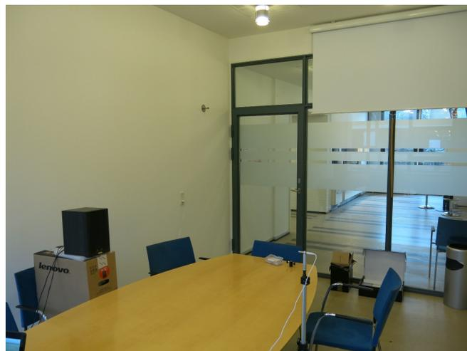
**Figure 1:** The meeting room with sound source and microphone on opposite side of the table.
