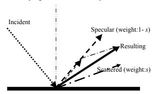
Figure 3: Vector based scattering. Reflecting a ray from a surface with a scattering coefficient of 50% results in a reflected direction which is the geometrical average of the specular direction and a random (scattered) direction. Note: Scattering is a 3D phenomena, but here shown in 2D.
