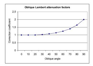
Figure 7: Correction factor for *Oblique Lambert*. When the oblique angle is zero, *Oblique Lambert* corresponds to traditional Lambert and the correction coefficient is one. When the oblique angle is 90° corresponding to grazing incidence on a smooth surface, the correction factor reaches its maximum of two.
