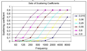
Figure 4: Frequency functions for materials with different surface roughness. The legend of each scattering coefficient curve denotes the scattering coefficient at 707 Hz.
