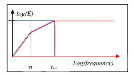
Figure 5: Energy reflected from a free suspended surface given the dimensions  $l \cdot w$ . At high frequencies the surface reflects energy specularily (red), at low frequencies, energy is assumed to be scattered (blue).  $f_w$  is the upper specular cut off frequency defined by the shortest dimension of the surface,  $f_l$  is the lower cutoff frequency which is defined by the length of the surface.
