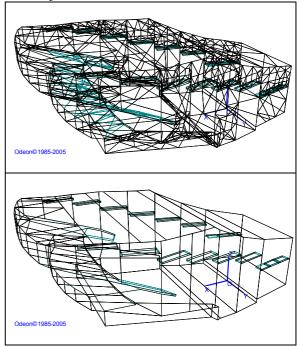
Figure 8: At the top a geometry which was imported from AutoCAD without stitching surfaces, at the bottom the model which was imported in ODEON using the stitching algorithm (Glue surfaces option). The number of surfaces was reduced from 869 to 115 surfaces without any additional user interaction forming a geometry compatible with the Reflection Based Scattering coefficient.
