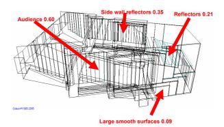
Figure 1: Example on combined scattering coefficients at 1000 Hz used in the Elmia hall, data was provided to participants in the 2<sup>nd</sup> Round Robin.
