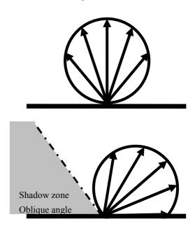
Figure 6: Traditional Lambert directivity at the top and Oblique Lambert at the bottom. Oblique Lambert produces a shadow zone where no sound is reflected. The shadow zone is small if scattering is high or if the incident direction is perpendicular to the wall. On the other hand if scattering is low and the incident direction is oblique then the shadow zone becomes large.
