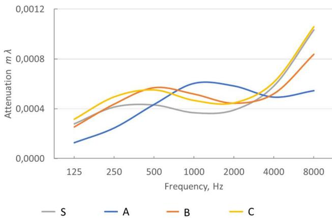
**Figure 4:** Air attenuation per wavelength as function of frequency. The curves represent different atmospheric conditions as during the measurements (A, B, and C) and for the standard atmosphere (S).
