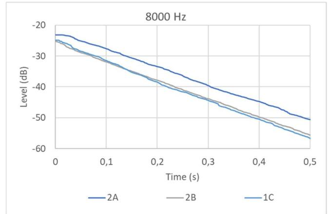
**Figure 9:** Decay curves measured at 8 kHz without normalisation. Measurements A with high humidity. Measurements B and C with low humidity.
