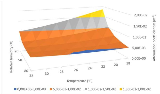
**Figure 3:** Air attenuation coefficient at 4 kHz and its variation with temperature and relative humidity.
