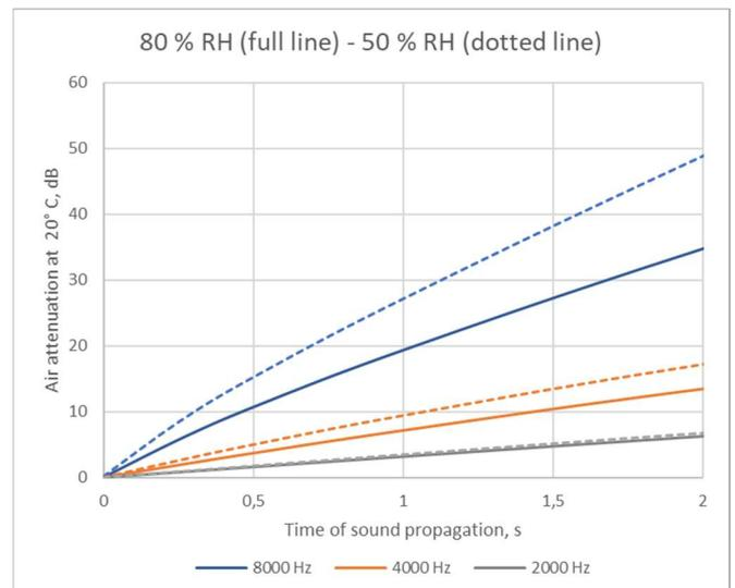
**Figure 6:** Air attenuation at 20 °C in octave bands up to 2 s propagation time. 80 % RH (full lines) and 50 % RH (dashed lines).
