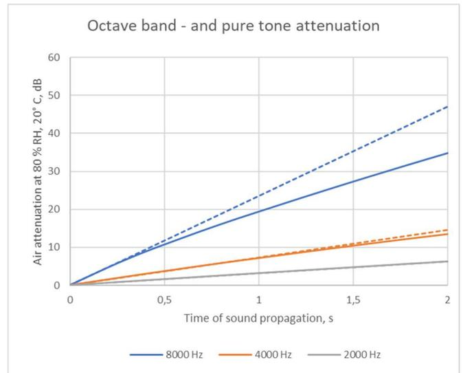
**Figure 5:** Air attenuation up to 2 s propagation time in very humid air. Octave bands (full lines) and pure tone centre frequency (dashed lines).
