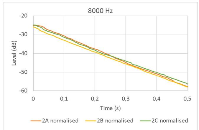
**Figure 10:** Decay curves at 8 kHz with normalisation to a standard atmosphere. Measurements A with high humidity. Measurements B and C with low humidity.
