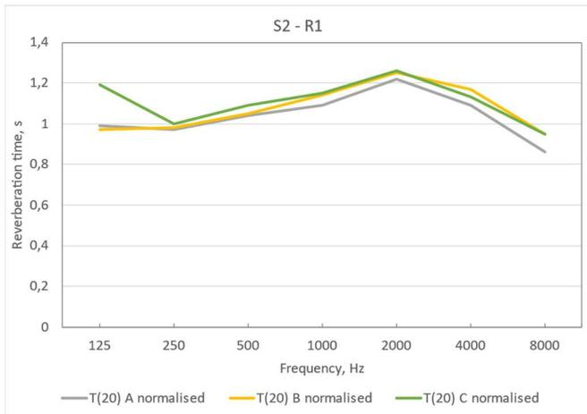
**Figure 8:** Reverberation time  $T_{20}$  in octave bands from 125 Hz to 8000 Hz normalised to a standard atmosphere. Results from three days A, B, and C.
