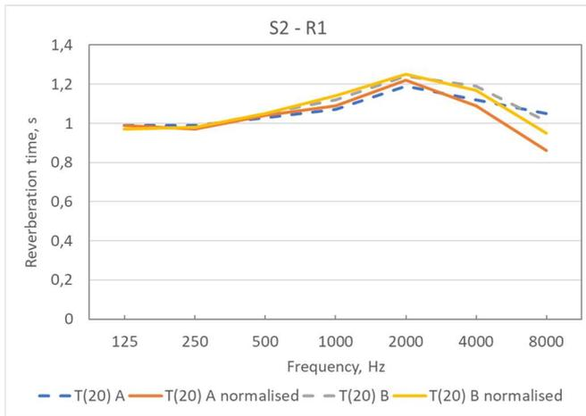
**Figure 7:** Reverberation time  $T_{20}$  as measured in octave bands from 125 Hz to 8000 Hz (dashed lines). Results normalised to a standard atmosphere (full lines). Measurements A with high humidity. Measurements B with low humidity.
