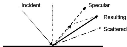
Geometrical weighting of specular and a scattered direction
