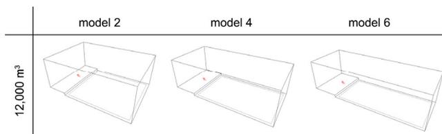
Fig.1 Three examples of simulated “shoe-box” halls in one of the analyzed volumes (V=12 000 m<sup>3</sup>). L/W ratio equals 1.43 (model 2); 2.10 (model 4); 2.77 (model 6).
