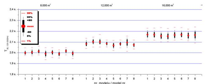
Fig.3 Room-averaged Reverberation Time  $T_{30, 125\sim 2000Hz}$  calculated by Odeon (grid response) in all analyzed volumes and models. Models N<sup>o</sup>. – see Fig.2.
