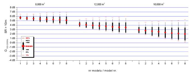
Fig.6 Comparison of room-averaged Strength  $G_{500-2000\text{Hz}}$  calculated by Odeon (grid response) in all analyzed volumes and models. Models N<sup>o</sup>. – see Fig.2.
