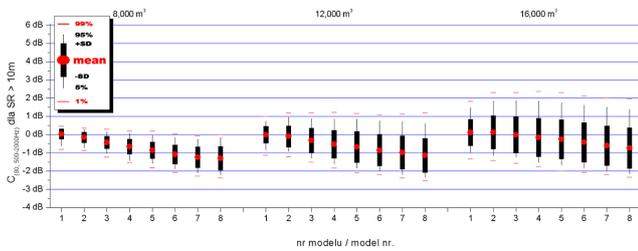
Fig.4 Comparison of room-averaged Clarity  $C_{80, 500-2000\text{Hz}}$  calculated by Odeon (grid response) in all analyzed volumes and models. Models N<sup>o</sup>. – see Fig.2.
