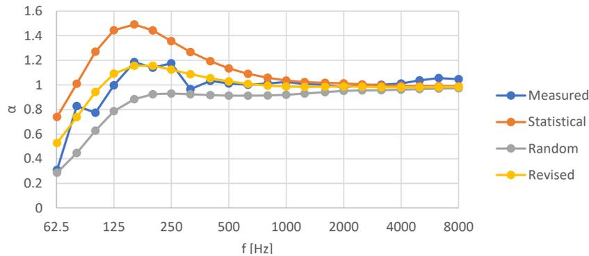
Figure 5. Measured and calculation absorption coefficients in a reverberation chamber (diffuse field). Rigid backing with 200 mm layer of polyester wool and mineral wool [8]. Statistical Eq. (10), Random incidence Eq. (9) and Revised Eq. (16).
