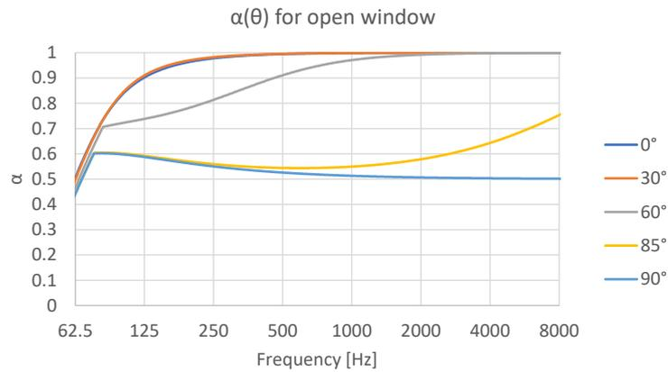
Figure 2. Angle-dependent absorption coefficient of an open window of dimensions 2 m by 2 m.
