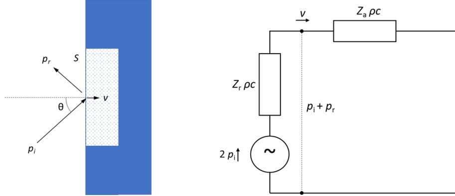
Figure 1. Reflection of a plane wave at oblique incidence on a finite-sized absorber flushed in a rigid backing. Left: sketch of the setup. Right: electrical analogue circuit.
