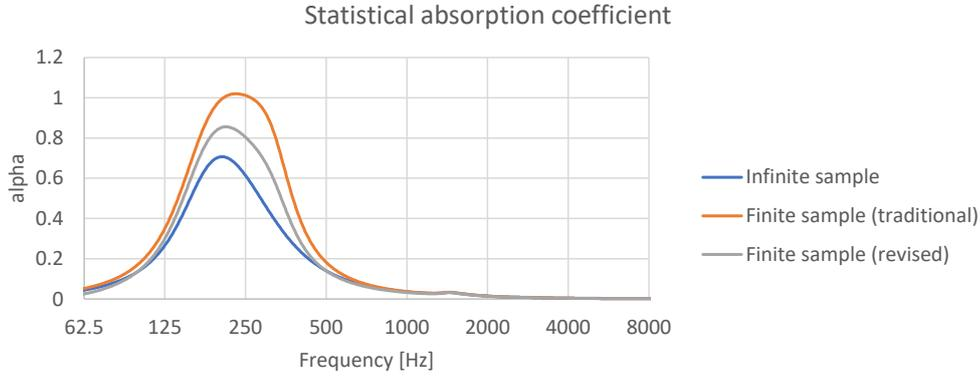
Figure 4. Statistical absorption coefficient. Comparison of the infinite sample calculation (blue), the traditional coefficient Eq. (10) (red) and the revised coefficient Eq. (16) (gray).
