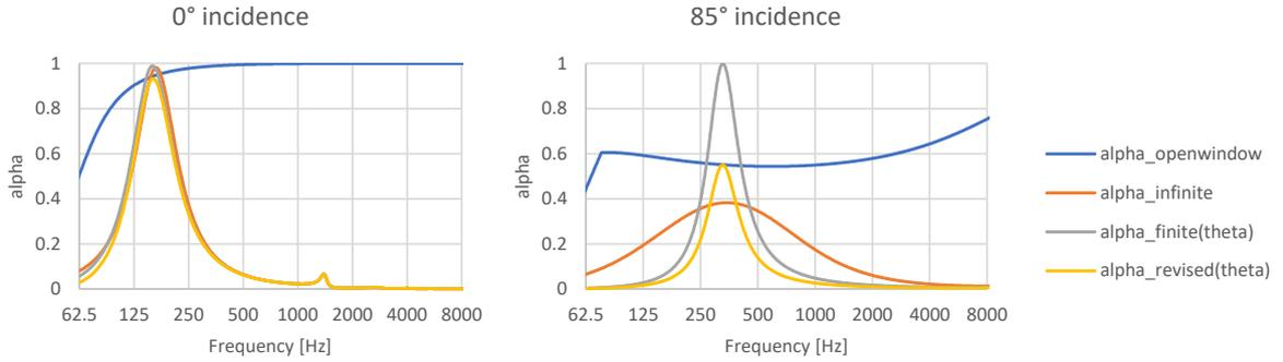
Figure 3. Angle-dependent absorption coefficients at  $0^\circ$  and  $85^\circ$  incidence. Comparison of the open window configuration Eq. (13) (blue), the infinite sample case Eq. (5) with  $Z_r$  from Eq. (3) (red), the original absorption coefficient for a finite sample Eq. (5) (gray) and the revised absorption coefficient Eq. (15) (yellow).
