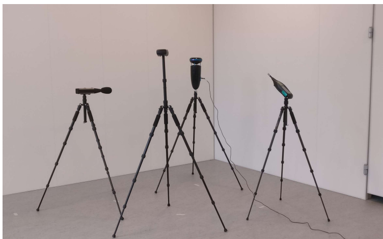
Figure 2: Picture of the experimental setup. Three sound level meters close to Source 2 (Odeon Omni).
