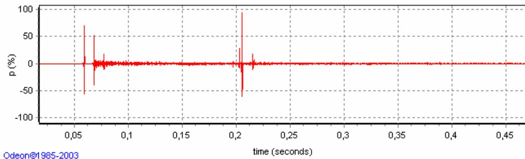
Figure 9 – Calculated impulse response in positions as in Figure 8. The echo is clearly seen.
