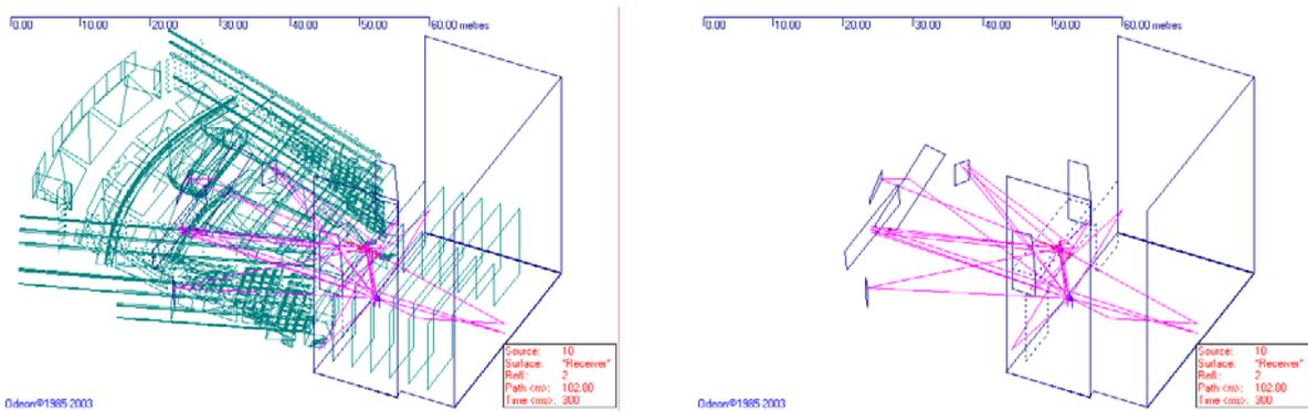
Figure 8 – 3D analysis of early reflections and possible echo problems from surfaces on the first balcony. Source is elevated 9,5 m above stage, receiver height 1,65 m. Right: Only reflecting surfaces are shown
