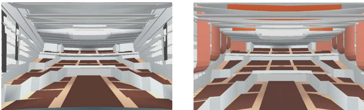
Figure 10 – Computer model of the final design, left: Opera configuration, right: Conference configuration with acoustic banners on walls and in the ceiling void.
