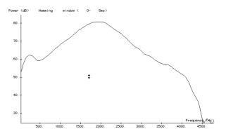
**Figure 14.** Frequency spectrum of the spark source (frequency axis is full scale).
