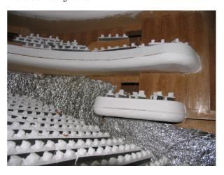
**Figure 29.** The scale model with sound diffusing treatment of the wall under the balcony.
