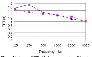
**Figure 21.** Average EDT with the source on stage. Blue triangles: Measured. Red squares: Simulated.
