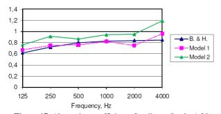
**Figure 17.** Absorption coefficient of audience for the 1:20 scale model compared to the Beranek & Hidaka data.
