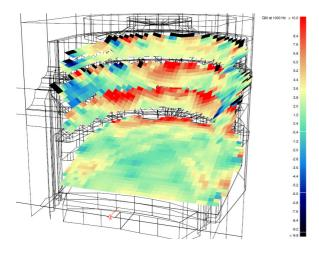
**Figure 10.** Grid response showing the Clarity C80 at 1 kHz. Source on stage.
