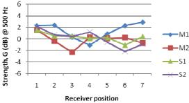
**Figure 27.** The Strength, G at 500 Hz in seven receiver positions. M1: measured, source on stage; M2: measured, source in the pit; S1 and S2: simulated, stage and pit positions.
