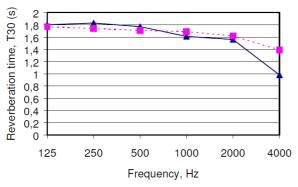
**Figure 20.** Reverberation time of the auditorium with the source in the pit. Blue triangles: Measured. Red squares: Simulated.
