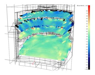
**Figure 9.** Grid response showing the Strength, G at 1 kHz. Source on stage.
