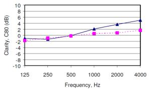
**Figure 26.** Average Clarity, C80 with the source in the pit. Blue triangles: Measured. Red squares: Simulated.
