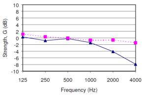
**Figure 24.** Average Strength, G with the source in the pit. Blue triangles: Measured. Red squares: Simulated.
