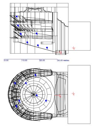
**Figure 1.** Section and plan of the digital model. The two source positions and the seven receiver positions are marked.
