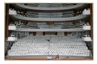
**Figure 12.** View into the auditorium of the 1:20 scale model. The spark source is seen on the stage in the front.
