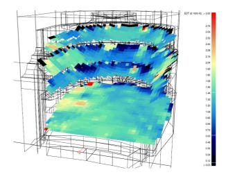
**Figure 8.** Grid response showing EDT at 1 kHz. Source on stage
