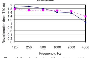
**Figure 19.** Reverberation time of the auditorium with the source on stage. Blue triangles: Measured. Red squares: Simulated.
