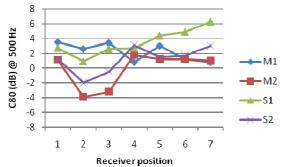
**Figure 28.** The Clarity, C80, at 500 Hz in seven receiver positions. Source positions as in Fig. 27.
