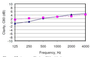
**Figure 25.** Average Clarity, C80 with the source on stage. Blue triangles: Measured. Red squares: Simulated.
