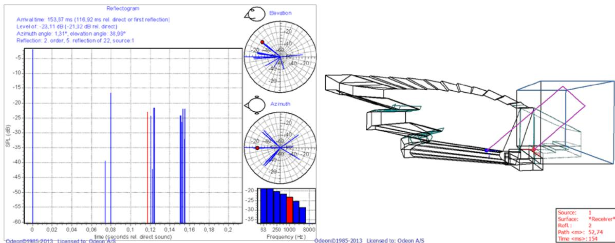
Figure 6 – Visualization of a sound reflection, left side as a line in a reflectogram and right side as a reflection path from source to receiver.
