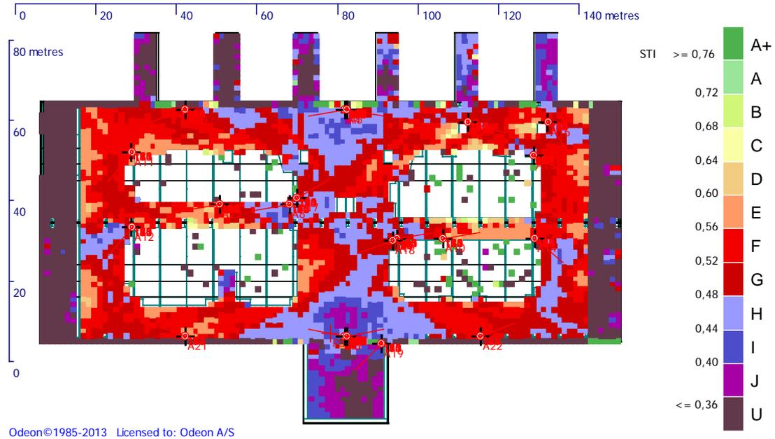
Figure 5 – Grid presentation of results using sharp separation of colors. The example shows the Speech Transmission Index calculated for a PA system in a railway station, applying the qualification bands as recommended in the standard.
