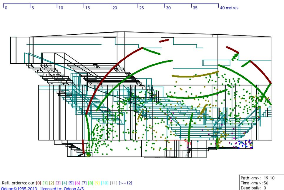
Figure 8 – Visualization of sound reflections as a large number of simultaneously emitted particles from a point source. The example shows a section in a concert hall.
