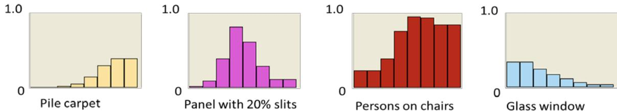
Figure 2 – Examples showing the absorption coefficients in eight octave bands (63 Hz to 8000 Hz) of four materials and the associated acoustic colors.
