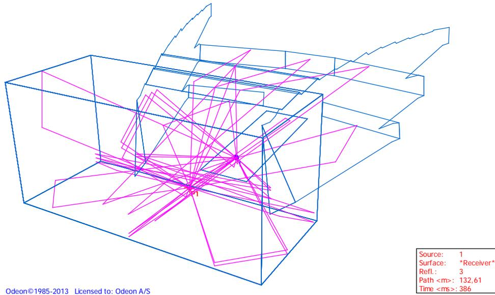
Figure 7 – Visualization of the reflection path from source to receiver of all reflections up to third order. Only the room surfaces creating reflections are shown here.
