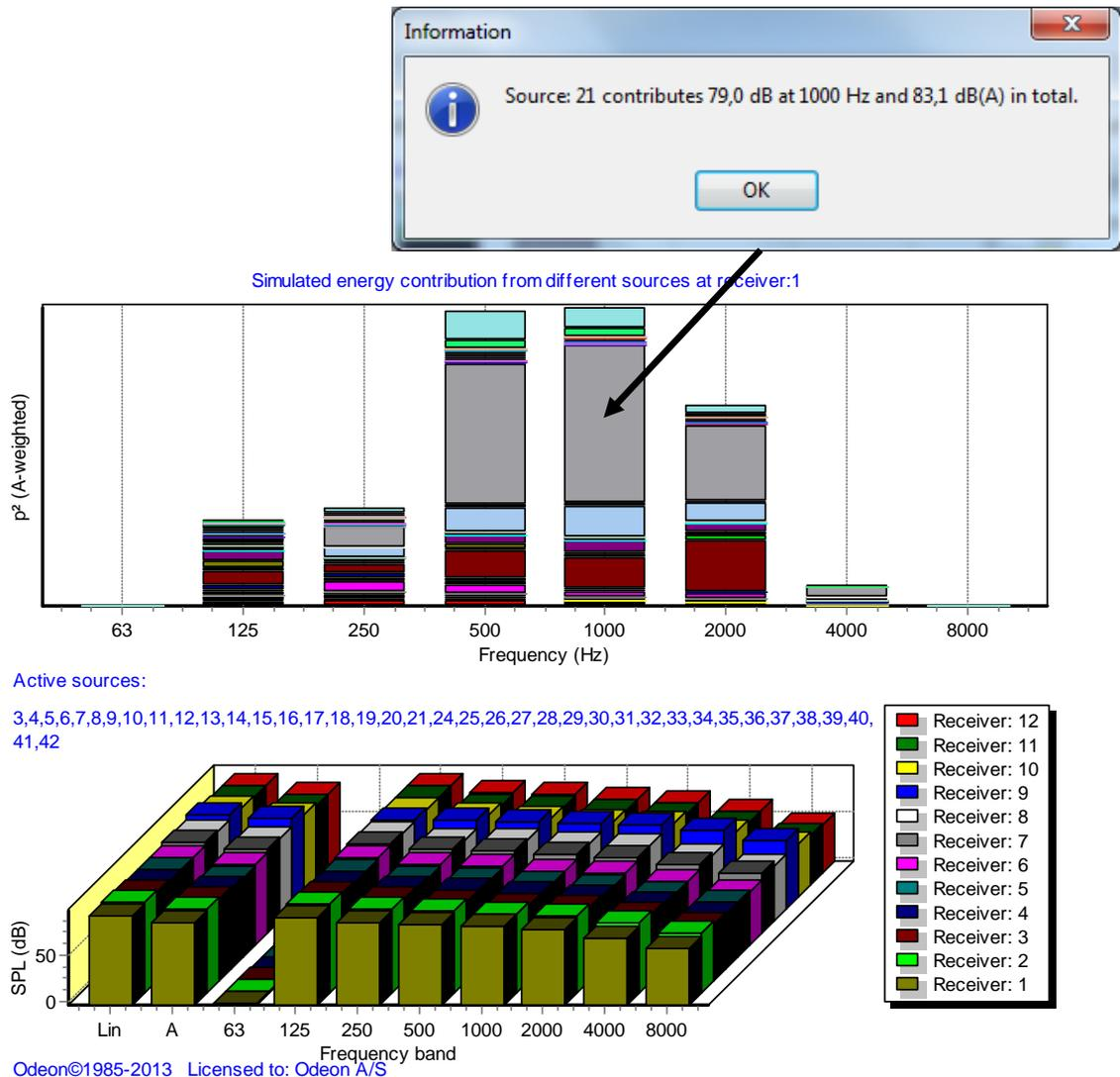
Figure 9 – Example of visualization of the relative contribution of many noise sources in a selected receiver point in a large industrial hall.
