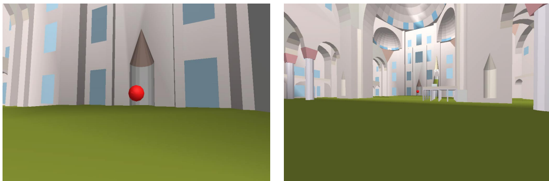
Figure 6: Odeon 3DOpenGL pictures of the Süleymaniye showing the source – receiver position. The picture is seen from the receiver position looking towards the source (dark dot).
