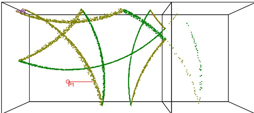
*Fig. 2. Visualization of the sound reflections shortly after an impulse. Some of the particles have been transmitted into the receiving room.*
