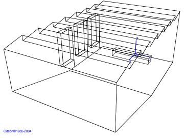
For some geometry it may be more appropriate to draw the geometries in one of the other main planes (XZ and YZ planes). As an example the auditorium.par model in the Figure has been modelled in the XZ plane, using separate extrusion surfaces for the room, the wall with windows holes, the table and the windows.
