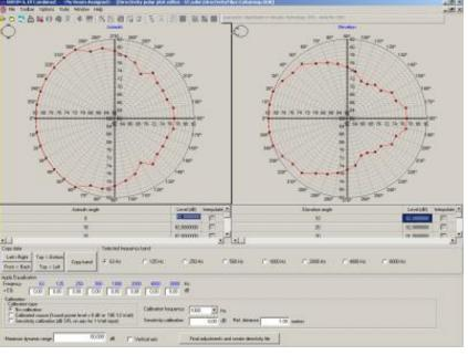
angles between the polar plots, ODEON will perform elliptical interpolation.
