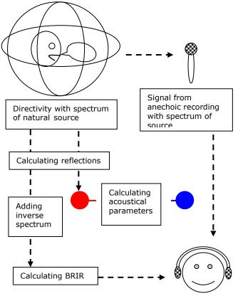
ODEON version 8.5 and later can manage to create correct estimates of parameters from natural sources and at the same time create correct auralisation, where the overall spectrum is only included once. But it is necessary to use a source marked natural:
