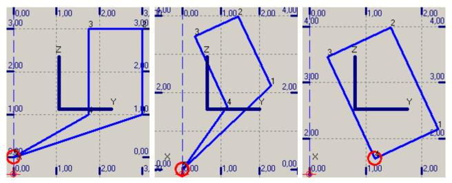
To rotate a surface around a point which is not included in the surface, a) Insert a rotation point in the surface, b) Use the Rotate surface shortcut Ctrl+R to activate the rotation dialog and specify the rotation angle – in this case 25 degrees, finally delete the rotation point from the surface.
