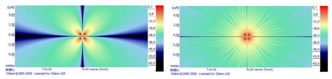
Figur E5 The Quadropol sample viewed in the Near filed balloon tab in the Array source editor. To the left at 63 Hz, to the right at 4 kHz.
