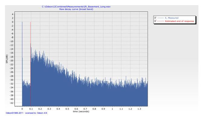
Fig. 12-7: An example of impulse response where the magnetic feedback from the recording system is very dominant. The feedback produces a sharp pulse before the actual start time of the impulse response. This pulse is wrongly detected as the start time of the impulse response and the estimated end is wrongly placed before the actual direct sound.
