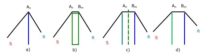
Figure 6-8. Diffraction paths and their detection. a) Odeon detects a 1 point diffraction path over a thin screen. b) Odeon detects a 2 point diffraction path over a wide barrier. C) Odeon fails to detect a diffraction path because the path from  $A_n$ - $B_m$  is obscured by a third surface – in fact it's a 3 point diffraction path. d) Odeon detects a diffraction path over two thin barriers.
