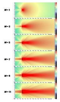
Figure 11-1. The radiation at 1 kHz from arrays with increasing number of units, from a single unit to 11 units (1, 3, 5, 7, 9 and 11).
