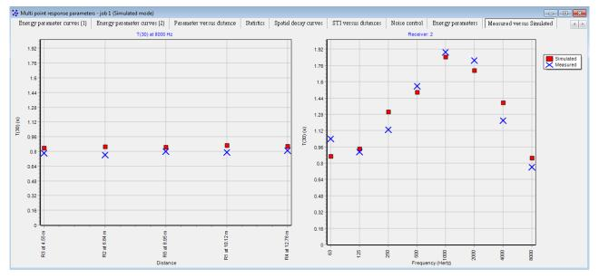
Fig. 12-2: Simulated and measured reverberation time  $T_{30}$  inside the Auditorium 21 at the Technical University of Denmark. The graph on the left shows the values at all receivers for a given octave band, while the graph on the right shows the values at all octave bands for a given receiver. Press the Up and Down arrows to change frequency. Press R to change receiver.
