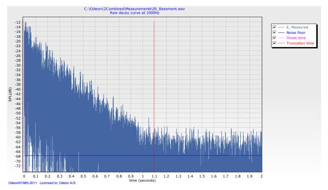
Fig. 12-3: Raw decay curve of a typical Impulse response with a well defined noise floor at the end of the impulse response. ODEON calculates the truncation time for each octave band individually. In this example the 1000 Hz filtered response is shown.
