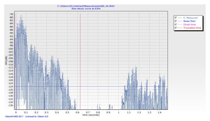
Fig. 12-10: Impulse response with a prominent hill at the end. Such a type of hill indicates that strong spikes were present during the measurement. When using the Sweep method, spikes in the recording are converted to hills after the deconvolution.
