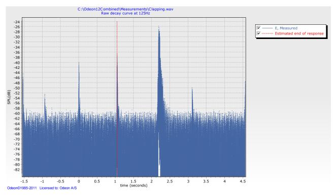
Fig. 12-6: Recording of Fig. 12-5 filtered at 125 Hz. The impulse response at this octave band has very poor peak to noise ratio and its length is too short, so that a truncation time is impossible to be derived. Instead, the estimated and of the response is displayed as an indication that the measurement is not trustful.
