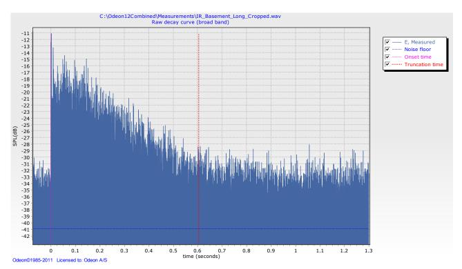
Fig. 12-9: Same impulse response as in Fig. 12-7. The pulse due to the magnetic feedback has been cropped away by the user.
