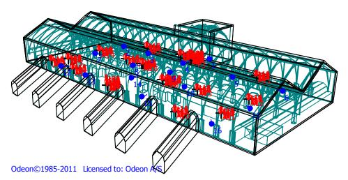
Copenhagen Central Station Array.par is available in the Auditorium and Combined editions of ODEON. This example demonstrates the newly installed PA system which utilizes 20 beam steered line arrays. Several measured parameters are available including STI. Creating new room models is probably the most time consuming task in room acoustical modelling. However good modelling practice will greatly reduce the time used for modelling and re-modelling rooms.
