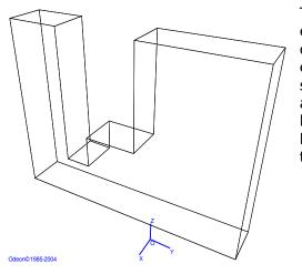
The Extrusion modeller allows modelling so called extruded geometries in a graphic environment – or in other words to draw geometries using the mouse. An extruded surface is a flat 2D outline, drawn at a specified drawing depth (the third coordinate) and with an extrusion height. When assigning an extrusion height to the 2D outline, it becomes a holster outlined by the edges of the 'extrusion surface', if so desired this holster can have a bottom and a top.
