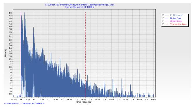
Fig. 12-11: Impulse response with prominent spikes at regular distances that indicate the presence of (flutter) echoes in the field between the buildings. The frequency is 4000 Hz.
