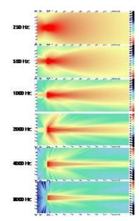
Figure 11-2. The radiation in octave bands from 250 Hz to 8 kHz for a line array with 7 units.
