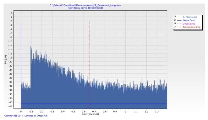
Fig. 12-8: Same impulse response as in Fig. 12-7. Now the Noise floor window length is set to 60ms. With this adjustment the estimated end of the response is placed correctly and a truncation time is derived. However, the onset time is still misplaced due to the magnetic feedback.
