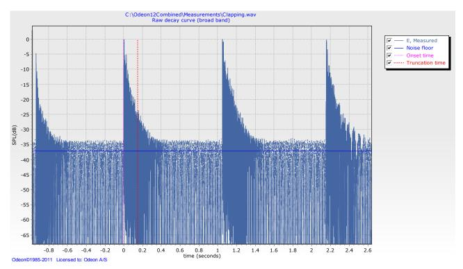
Fig. 12-5: An example of recording that contains four impulse responses in a row. Hand claps have been used for excitation. ODEON detects the second impulse response as being the strongest one and sets an onset and a truncation time for it. Calculation of the onset time is performed on the broadband signal as suggested in ISO 3382-1, A.3.4 and not for each Octave band separately.
