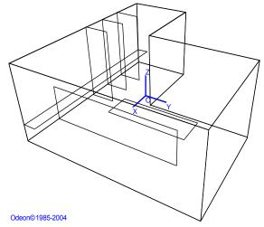
In the extrusion modeller it is possible to make one drawing which contains multiple extrusion surfaces, each described by a 2D outline (a simple drawing) and the line properties; drawing depth, extrusion height, bottom check mark, top check mark and a name. If the extrusion is created in the XY- plane, then one extrusion surface may form a volume with walls and optional floor and ceiling, whereas other extrusion surfaces define tables, chairs or screens.
