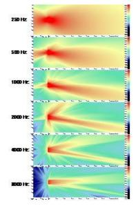
Figure 11-4. The radiation in octave bands from 250 Hz to 8 kHz for a line array with 7 units and a time delay 0,1 ms per unit.
