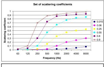
Figure 6-3: Frequency functions for materials with different surface roughness. The legend of each scattering coefficient curve denotes the scattering coefficient at 707 Hz.
