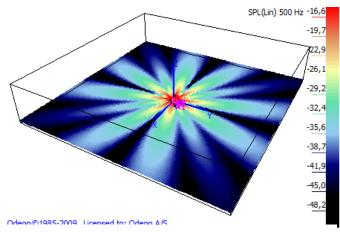
Figur E4 The Quadropol directivity pattern viewed in the 3D\_Direct display at 500 Hz. Because the distances between the transducers are 1 metre, the Quadropol pattern has broken down at 500 Hz. Frequency dependent and have pronounced symmetry properties; At high frequencies their patterns break down and show strong fluctuations (see figure E4), and viewing an Octopol in the Near field balloon display may not
