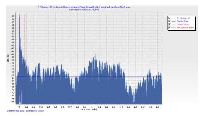
Fig. 12-4 Impulsive noise has been present when the impulse response was measured. If Signal to noise ratio is insufficient to derive all room acoustics parameters or if you are suspicious that there may be strong hills or spikes polluting the impulse response, then try to repeat the measurement under more quiet conditions, with an output gain or with a longer sweep length.
