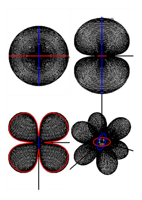
Figure E3 Images of the Mono, Dipol, Quadropol and Octopol directivity patterns installed with Odeon Auditorium and Combined, as viewed in the Far field balloon tab in the Odeon Array Source Editor.
