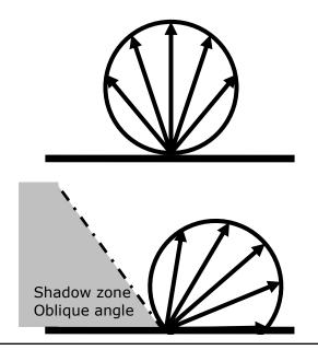
Figure 6-6. Traditional Lambert directivity at the top and Oblique Lambert at the bottom. Oblique Lambert produces a shadow zone where no sound is reflected. The shadow zone is small if scattering is high or if the incident direction is perpendicular to the wall. On the other hand if scattering is low and the incident direction is oblique then the shadow zone becomes large.
