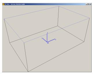
The Unique Edges option in the 3DView display shows edges, which only occur on one surface. Such an edge is "free"; it might be the edge of a free-hanging reflector, but it also could be the result of an error whereby two surfaces, which should join along an edge, do not.
