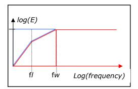
Figure 6-4. Energy reflected from a free suspended surface given the dimensions I.w. At high frequencies the surface reflects energy specularily (red), at low frequencies, energy is assumed to be scattered (blue). fw is the upper specular cut off frequency defined by the shortest dimension of the surface, fl is the lower cutoff frequency which is defined by the length of the surface.
