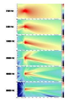
Figure 11-7. The radiation in octave bands from 250 Hz to 8 kHz for a line array with 7 units. The time delay is 0,1 ms per unit and the level increases by 2 dB per unit from bottom to top.
