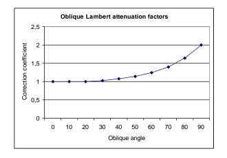
Figure 6-7. Correction factor for *Oblique Lambert*. When the oblique angle is zero, *Oblique Lambert* corresponds to traditional Lambert and the correction coefficient is one. When the oblique angle is 90° corresponding to grazing incidence on a smooth surface, the correction factor reaches its maximum of two.
