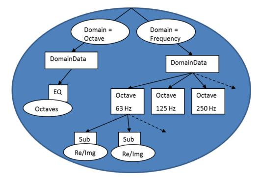
Figure E2. Tree structure with the details of the Domain Data node. This note comes in two versions depending on weather Domain=Octave or Domain=Frequency.
