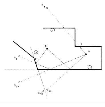
Figure 6-1. Visible and invisible images. Images S1 and S21 are visible from R, while S2, S3 and S12 are not.
