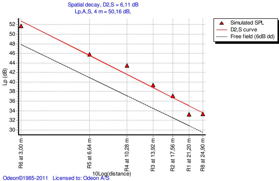
Figure 2. Spatial decay of A-weighted SPL in office 3, measurement line 2. Note the logarithmic distance scale.
