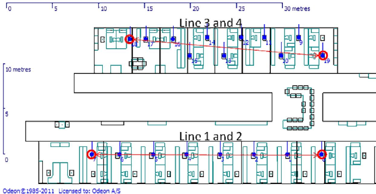
Figure 1. Plan of office with source and receiver positions. Four measurement lines are used, each associated with a point source.
