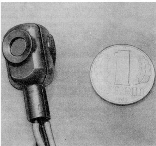
Fig. 4. Dummy head with two microphones in scale 1:20. ([10] fig. 9.69).
