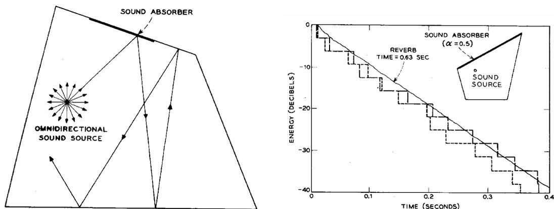
Fig. 6. Particle tracing based on geometrical acoustics. Left: The sound energy follows the path of several hundred rays (only one is shown), and the energy of the particles is reduced when they hit an absorbing surface. Right: Average decay curve. (After Schroeder [17]).
