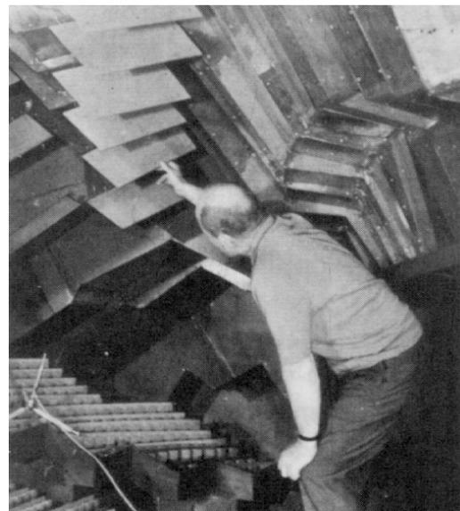
Fig. 5. View from a 1:10 scale model of the Major Hall for the Sydney Opera House (not the final design, but the last Utzon design around 1966). ([11] fig. 4.10).
