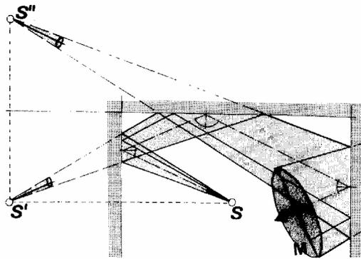
Fig. 8. Tracing of a circular cone from the source S to the receiver M. The first and second order image sources are also shown. ([21] fig. 2).
