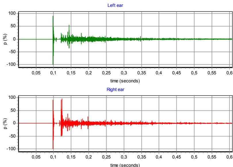
Fig. 9. Example of a Binaural Room Impulse Response calculated in a new opera house project. The first 600 ms are shown, but in this example the calculated impulse response is 2 s long.
