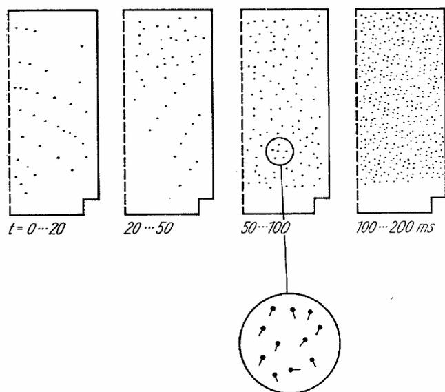
Fig. 7. Example of results from the first ray tracing model [18]. Hit points of sound rays as distributed on one half of the floor, shown in time intervals relative to the direct sound. Some directional information is included, see the enlargement.
