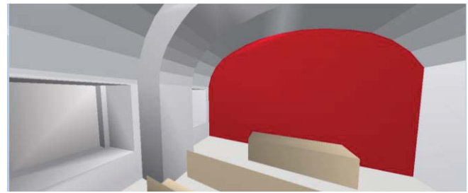
Figure 16. Classroom render by Odeon software, with absorbent panels (red surface) behind the teacher position.
