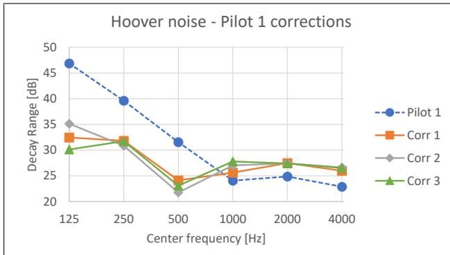
**Figure 7.** Measured decay range for sweeps corrected from the first pilot in hoover conditions.
