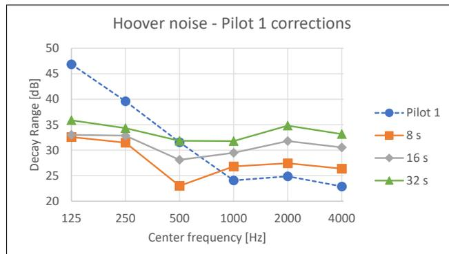
**Figure 8.** Decay range of corrected sweep measurements with different sweep lengths in hoover noise conditions.
