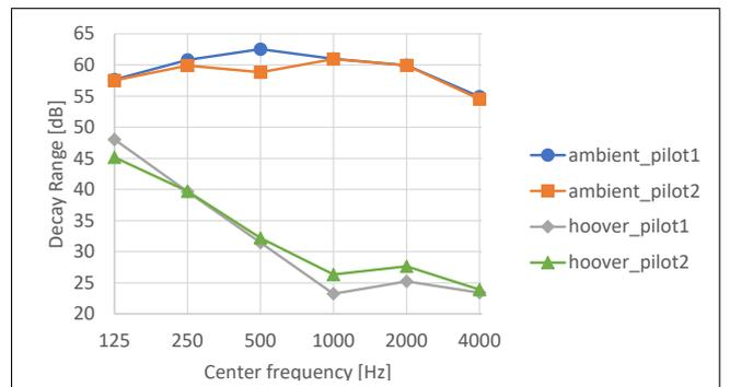
**Figure 5.** Measured decay range for pilot measurements of 8 s in ambient and hoover conditions.
