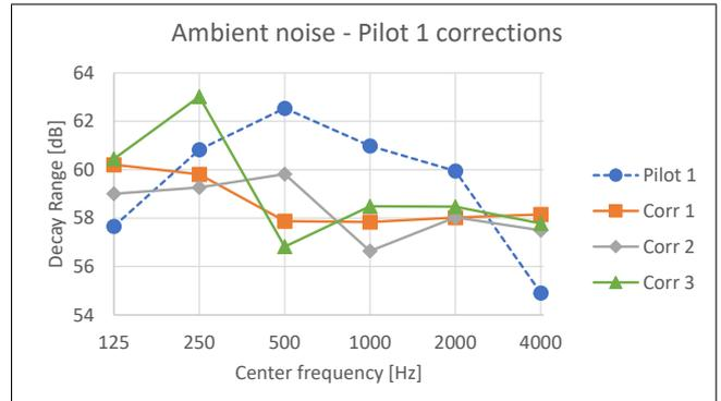
**Figure 6.** Measured decay range per octave band for sweeps corrected from Pilot 1 in ambient conditions.
