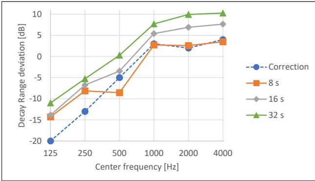
**Figure 9.** Decay range deviation from Pilot 1 for different sweep lengths in hoover noise conditions.
