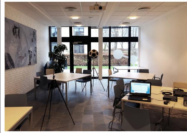
**Figure 3.** Measurement setup in a meeting room. Room dimensions 5 m × 9.3 m × 2.9 m.
