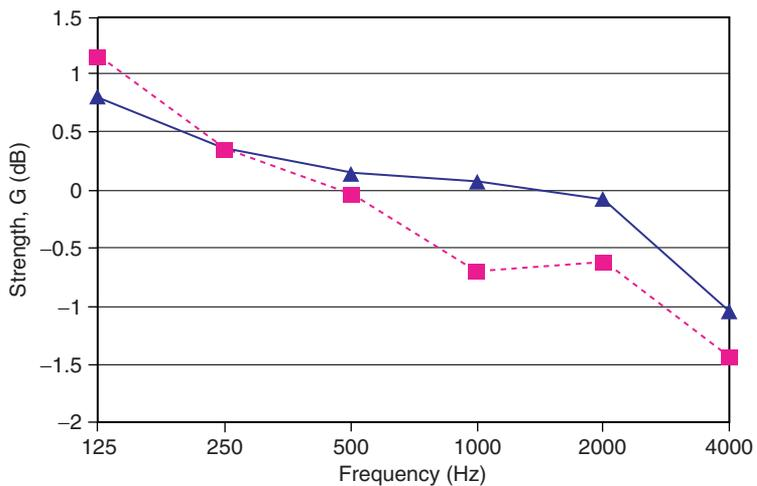
Figure 5. Average Strength, G. Blue triangles: Source on stage. Red squares: Source in pit.
