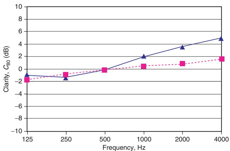
Figure 26. Average Clarity,  $C_{80}$  with the source in the pit. Blue triangles: Measured. Red squares: Simulated.
