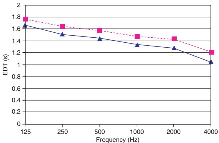
Figure 4. Average EDT. Blue triangles: Source on stage. Red squares: Source in pit.
