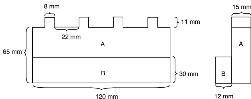
Figure 15. Schematic drawing of 1:20 model audience.
