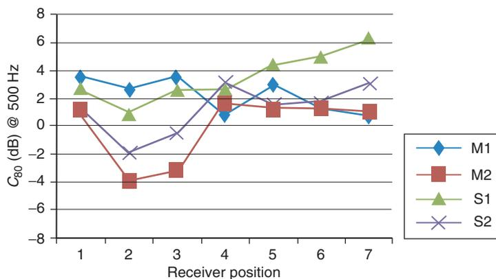
Figure 28. The Clarity,  $C_{80}$ , at 500 Hz in seven receiver positions. Source positions as in Fig. 27.
