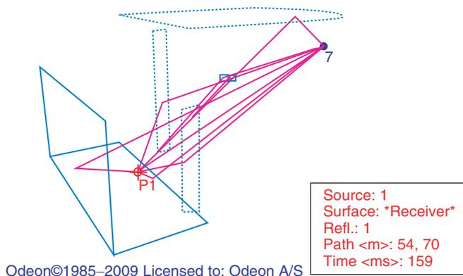
Figure 30. Example of an analysis in 3D of the reflection paths of early reflections.
