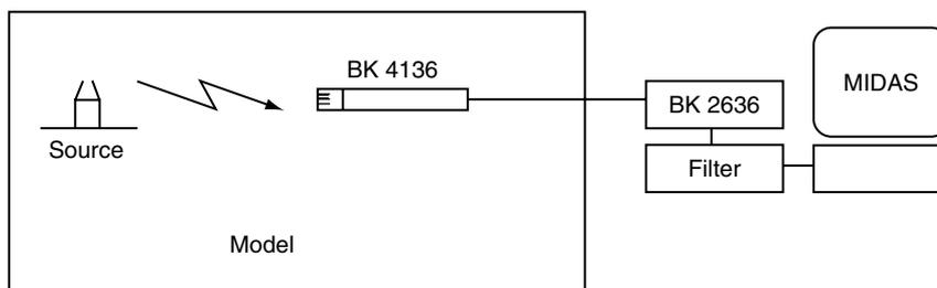
Figure 13. Setup for scale model measurements.
