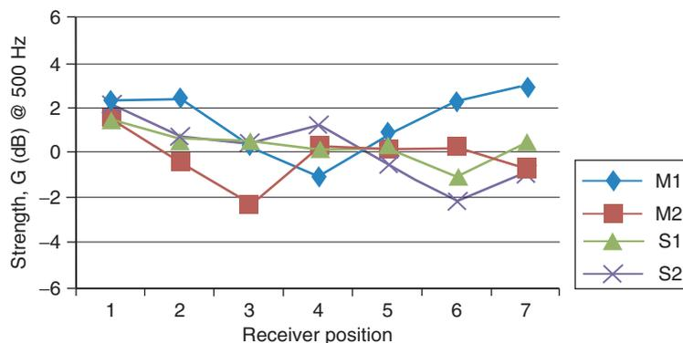
Figure 27. The Strength,  $G$  at 500 Hz in seven receiver positions. M1: measured, source on stage; M2: measured, source in the pit; S1 and S2: simulated, stage and pit positions.
