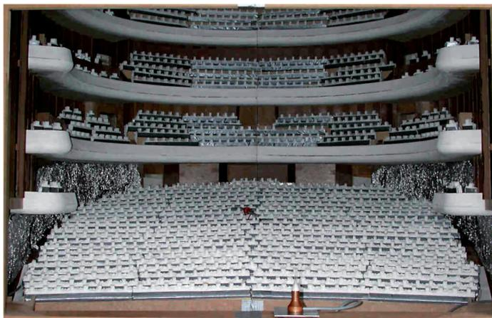
Figure 12. View into the auditorium of the 1:20 scale model. The spark source is seen on the stage in the front.
