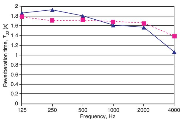
Figure 19. Reverberation time of the auditorium with the source on stage. Blue triangles: Measured. Red squares: Simulated.
