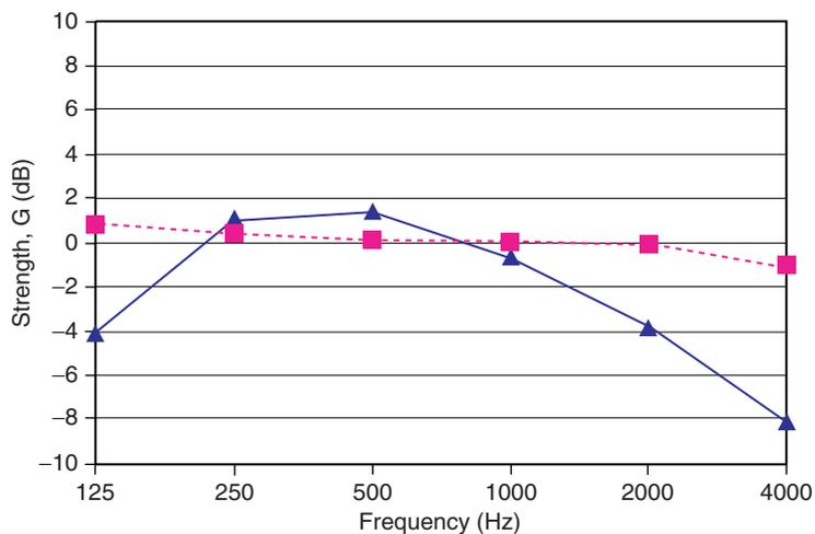
Figure 23. Average Strength, G with the source on stage. Blue triangles: Measured. Red squares: Simulated.
