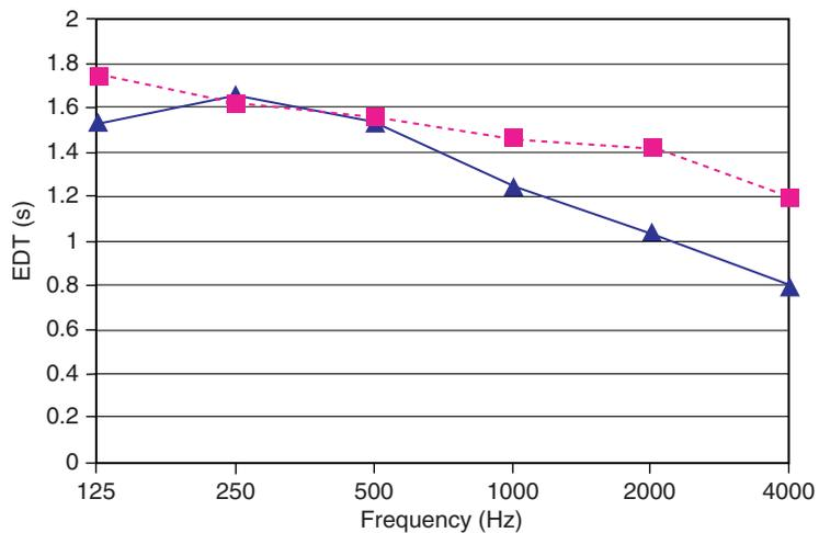
Figure 22. Average EDT with the source in the pit. Blue triangles: Measured. Red squares: Simulated.
