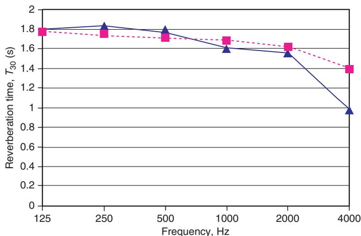
Figure 20. Reverberation time of the auditorium with the source in the pit. Blue triangles: Measured. Red squares: Simulated.
