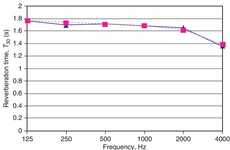
Figure 3. Average reverberation time. Blue triangles: Source on stage. Red squares: Source in pit.
